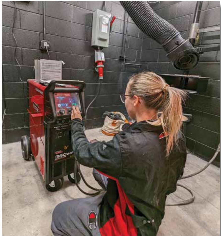
Above: New welding lab booths feature the latest Lincoln welders and air handling equipment. Below: Manufacturing Tech Instructor Andrew Paad (middle) works with students on one of the robotic arm trainers.
